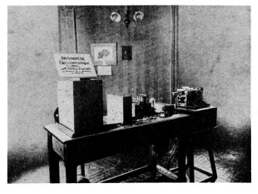
Annals of the History of Computing Vol. 2, No. 3 July 1980 **31** Torres y Quevedo Machine A fundamentally different type of division control was developed by Torres y Quevedo of Madrid. He built an electromechanical machine and exhibited it at the Paris Centennial of 1920. This machine is typewriter controlled.
