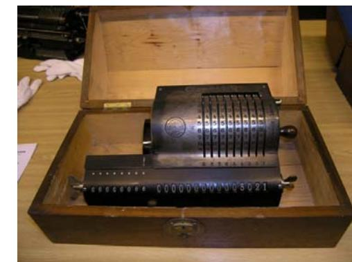
**Figure 19.** Odhner-Hill arithmometer nr. 1148 of the National Museum of Science and Technology, Stockholm in an original case. This is the first known 15-digit model. The coverplate here is nickelplated, which was at that time cheaper than a lacquered coverplate [86], see also Figure 21.
