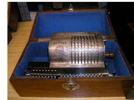
**Figure 17.** Odhner arithmometer nr. 852 (capacity 13) at the National Museum of Science and Technology, Stockholm. This calculator was produced in January 1892 and is the gift of the inventor to Crown Prince Gustaf.
