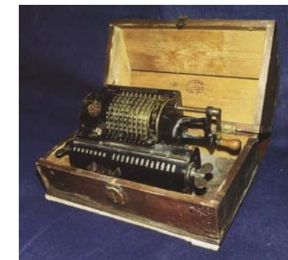
**Figure 20.** Odhner-Hill arithmometer nr. 1326 of Sergei Frolov, photo ©Sergei Frolov. The case is original, but the long crank, decimal pointers and input lever clearing system have evidently been refurbished later. The number wheels here (as in arithmometer nr. 1209) have black numbers on a white background.
